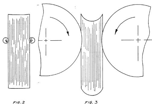
If, on the other hand, the rollers were to have a very large diameter, such as shown in exaggeration in figure 3, then the surface area for the rollers gripping the volume is large, displacement will be positive and a true concave/convex shape would result. However, having a very large diameter-rounding roller presents severe design limitations. The result is a roller with a compromised diameter that would be suitable for a great percentage of the work in the bindery, but not for 100%.
