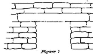
The simple old lintel was used in ancient times before a better understanding of architectural structure was common. Bridges were once just logs laid across a stream. We do not find many examples of bridges constructed with the lintel principle at the present time, for obvious reasons.
