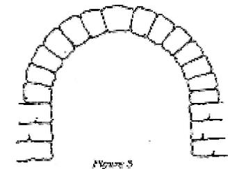
The rest of the bricks can be laid around and over the arch. One can readily see that the stones cannot slide down and fall because they are like wedges. The top stone of the arch, which is called the keystone, tries to slide down but cannot do so without forcing apart the stones on each side of it, known as the voussoirs. Its downward push is changed to a sidewise thrust against the stones next to it and these carry the thrust to the next stones, and so on down around
